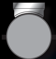
Type ZDE Is fitted in the suspended ceiling outside the door system and distributes airflow evenly along the door opening.
