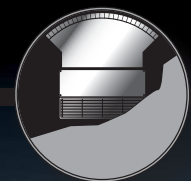
Type SDE Is fitted into the canopy of the revolving door and distributes airflow evenly along the door opening.
